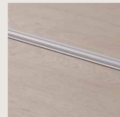
MULTIFUNCTIONAL PROFILE SILVER 1860 × 47 × 16 mm The Pergo multifunctional profile can level height differences for a smooth transition onto any other type of floor. Suitable for height differences of 0 – 12,3 mm. Surface: aluminium. PGPRSILV
